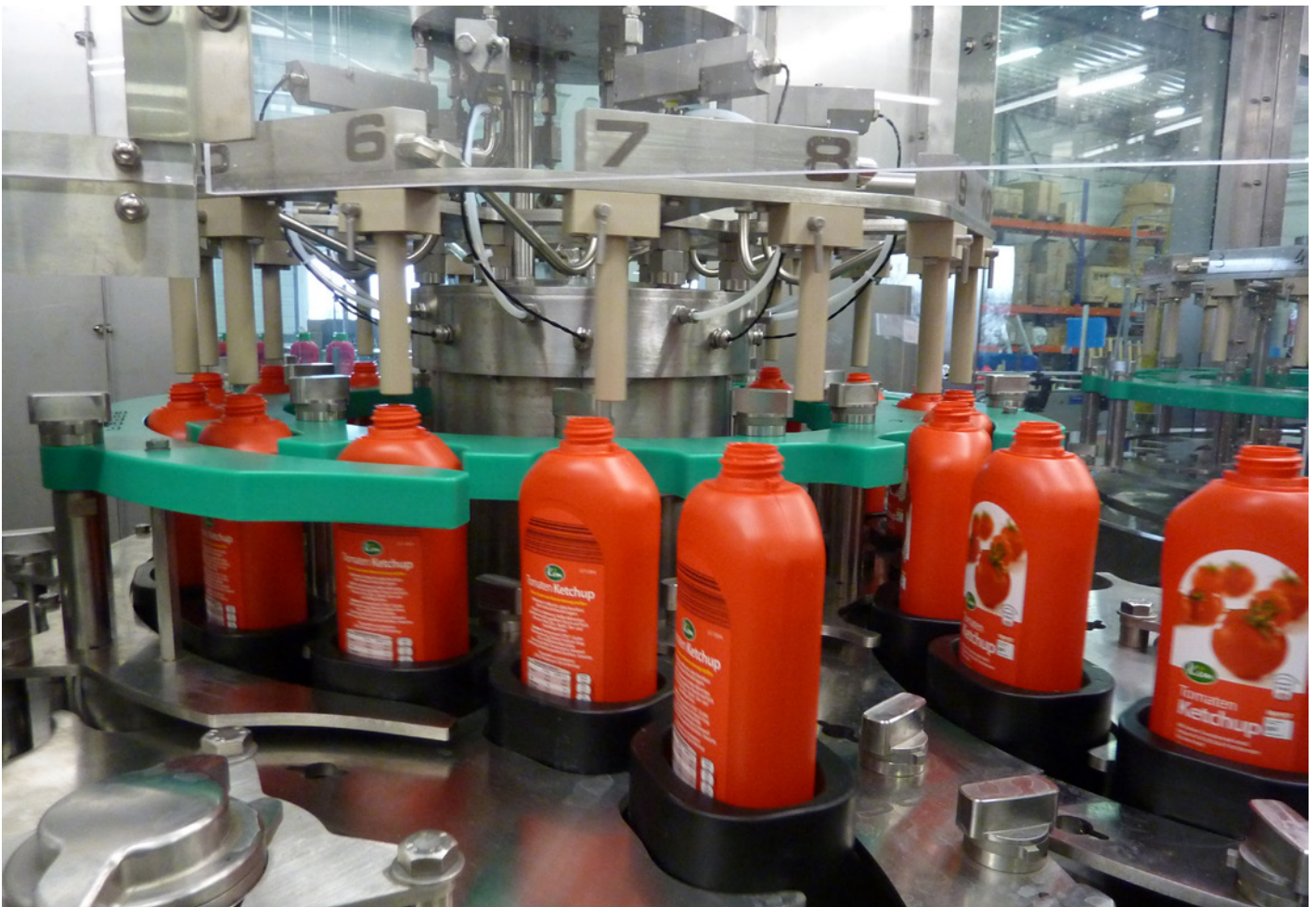
Figure 2: Dry decontamination of the packaging just before weight filling
