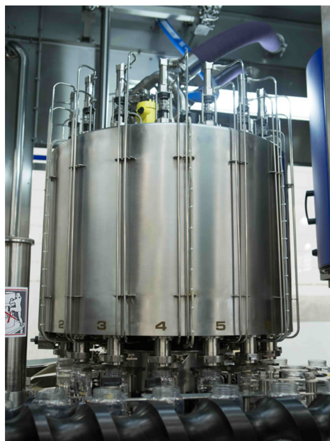
Figure 1: Weight filling assisted by overpressure for highly viscous products
